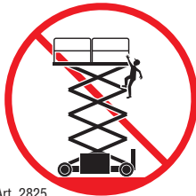
Art_2825 DO NOT EXIT PLATFORM WHEN ELEVATED
